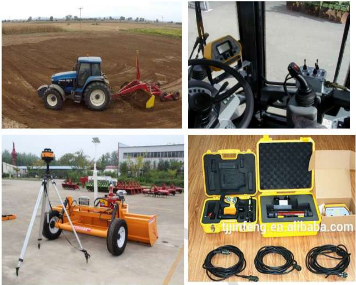
Figure 3. Laser land leveler and its components
